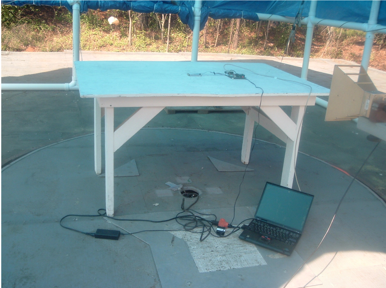
Photo 6. Above 1GHz Test setup at 1 meter
