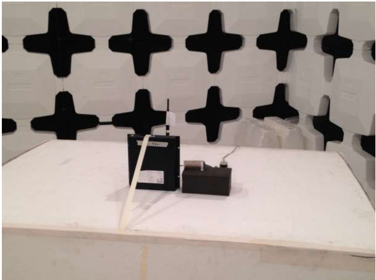
Figure 1. EUT w/Dipole Antenna, Intentional Radiated Emissions Setup
