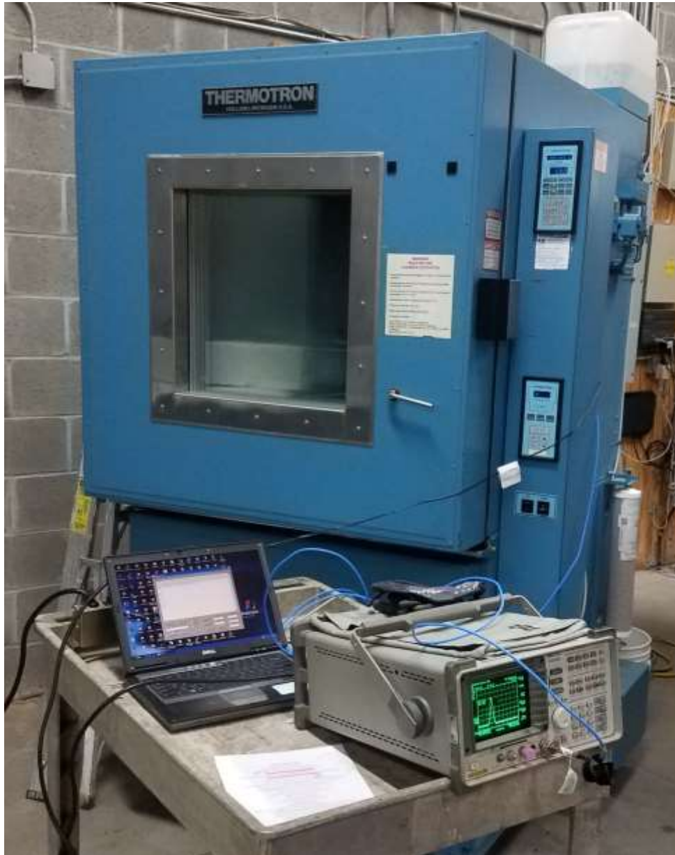
Figure 12. Frequency Stability testing, Temperature Chamber Setup
