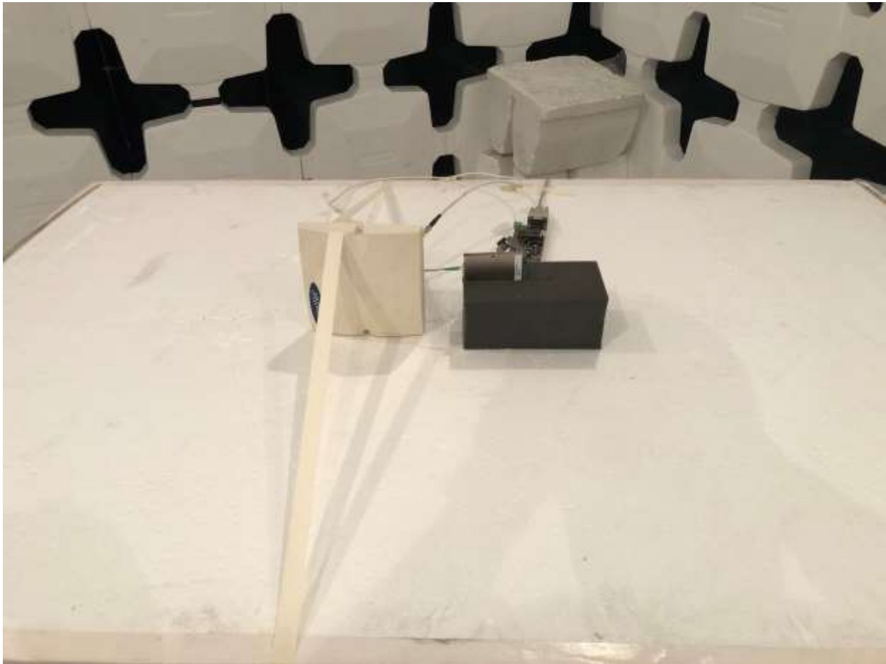
Figure 4. EUT w/Patch Antenna, Intentional Radiated Emissions Setup
