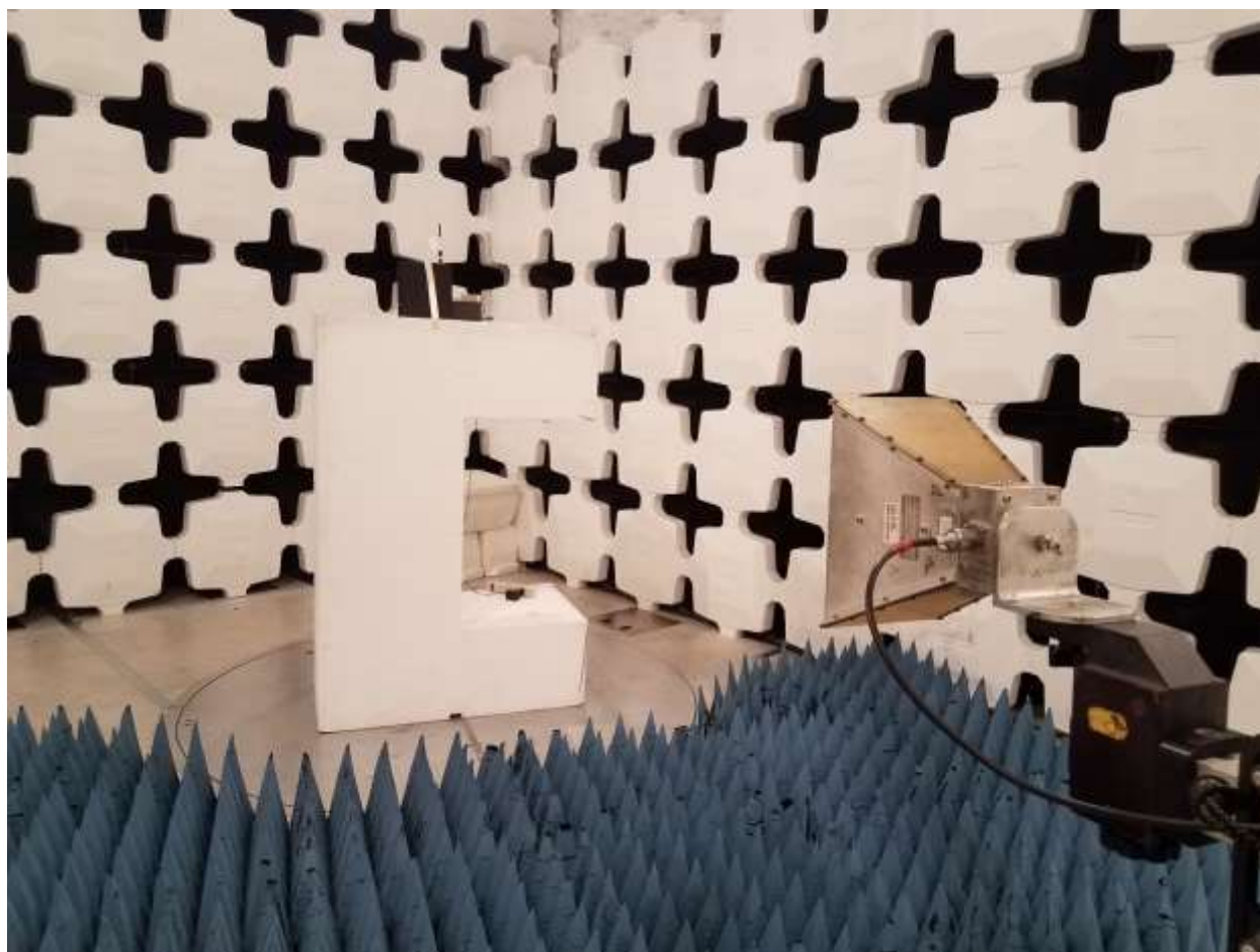
Figure 3. EUT w/Dipole Antenna, Harmonics Emissions Setup
