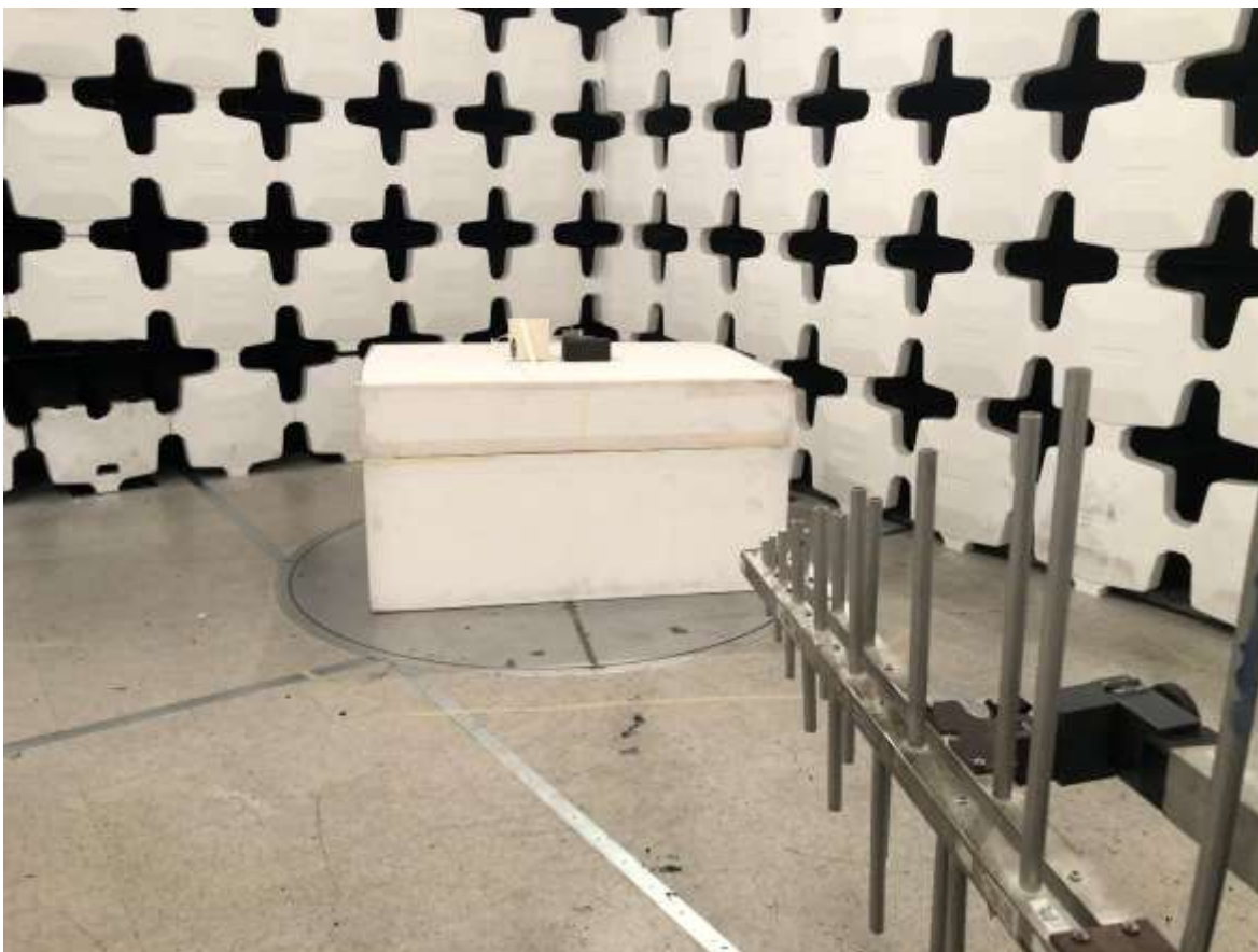
Figure 5. EUT w/Patch Antenna, Fundamental Emissions Setup
