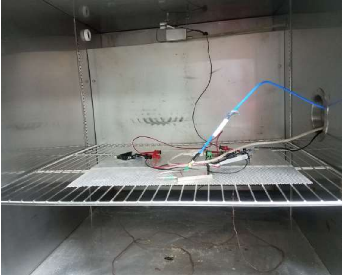
Figure 13. Frequency Stability, Radio Module within the Chamber
