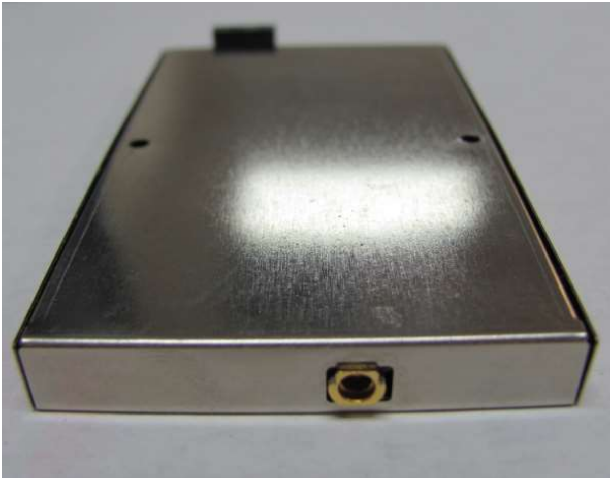
Figure 3: EUT Front – Antenna Connection Port
