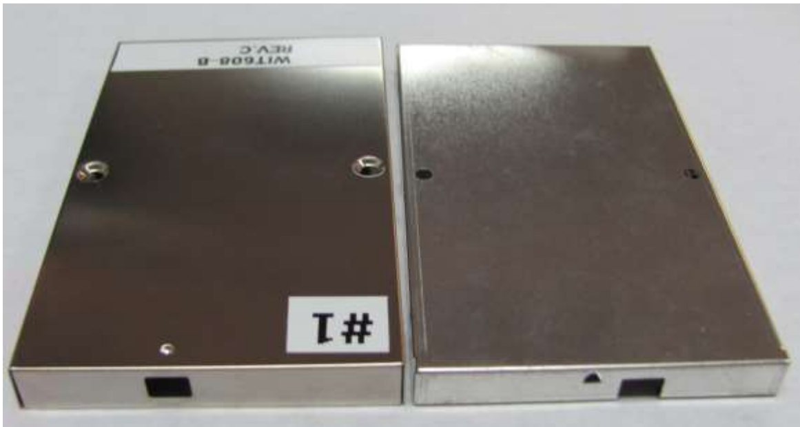
Figure 9: RF Module Shield, Empty
