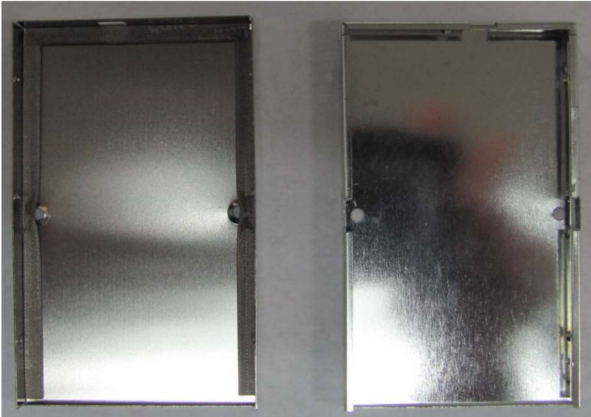
Figure 8: RF Module Shield – Internal
