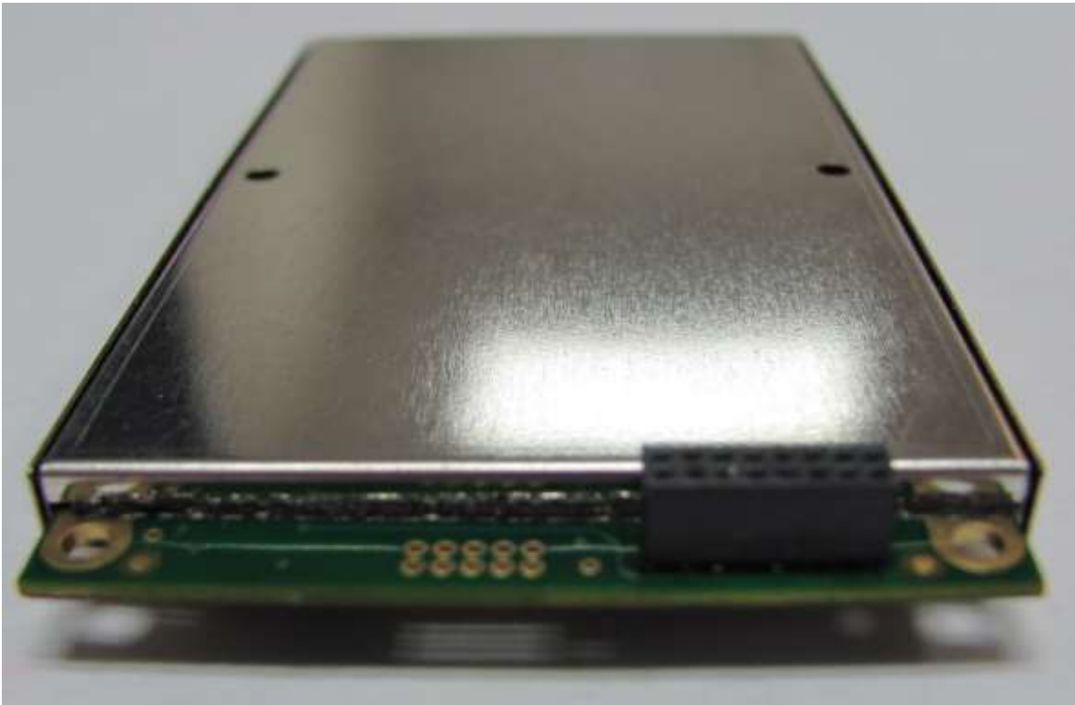
Figure 4: EUT Back – Connection to the Main PCB Board
