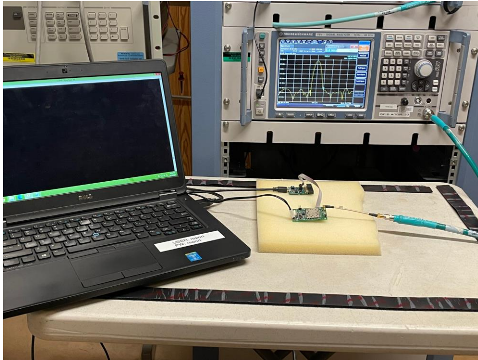
Figure 1: Equipment Under Test – Antenna Port Conducted measurements Note: RF Conducted Measurements were only performed to evaluate the Bandwidth.
