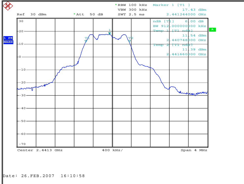
Figure 7.4.2-2: 6dB Bandwidth Plot – Mid Channel
