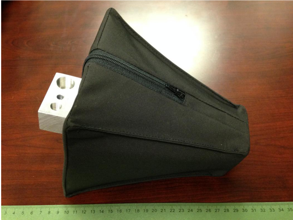
Figure 3. CP Beam Antenna View 3
