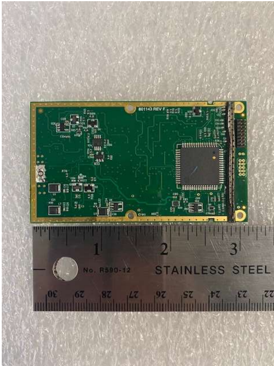
Figure 2. Radio with Shield Removed - Bottom
