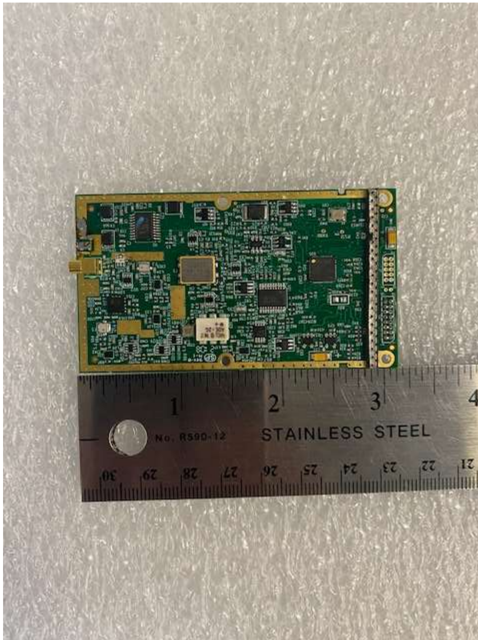
Figure 1. Radio with Shield Removed – Top
