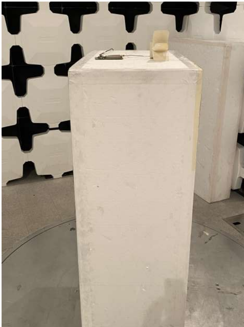
Figure 1. Radiated Emissions, EUT Worst Case Position Test Setup: EUT with Corner Reflector Antenna
