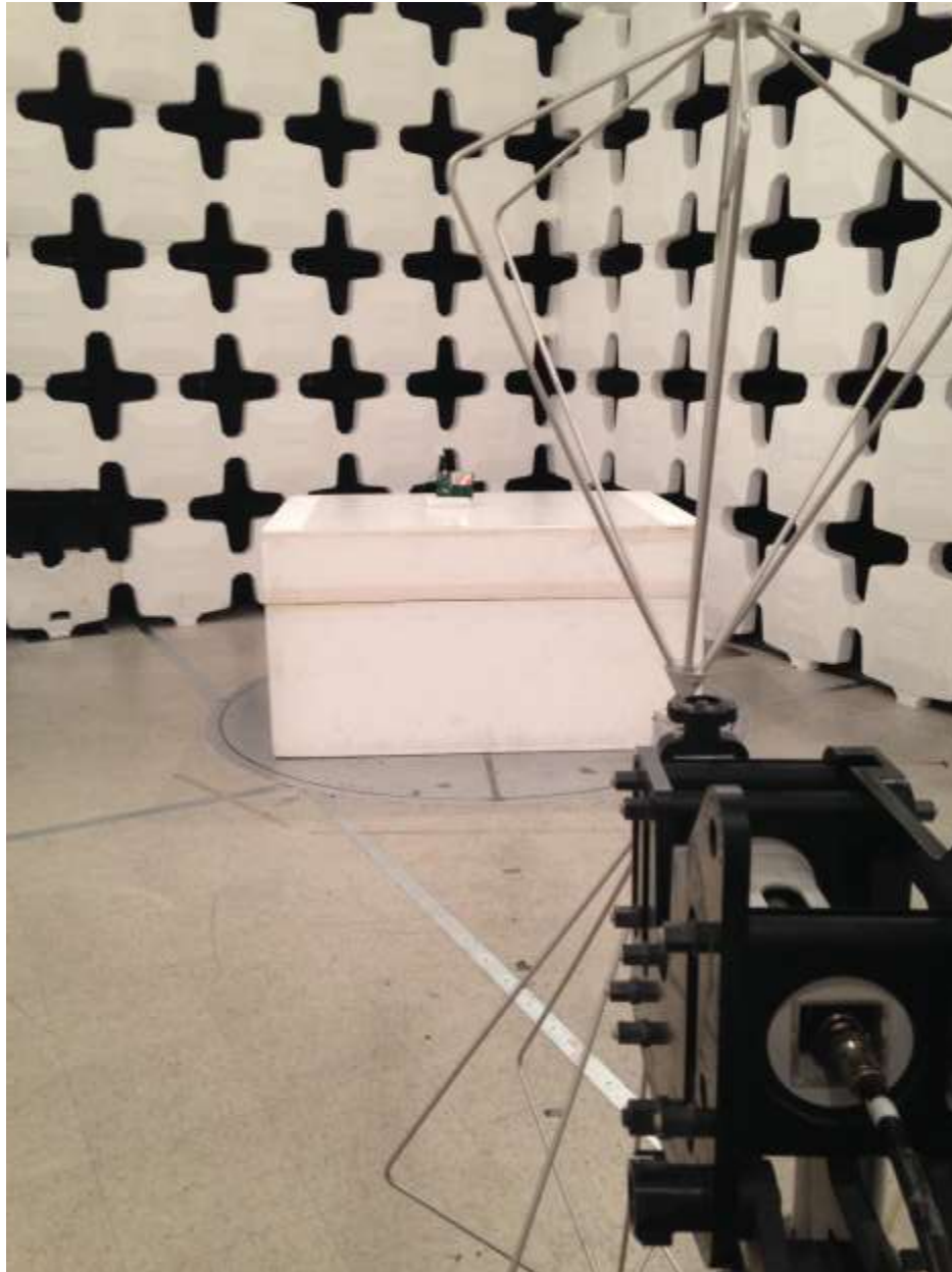
Figure 9. Radiated Spurious Emissions: 30 MHz to 200 MHz
