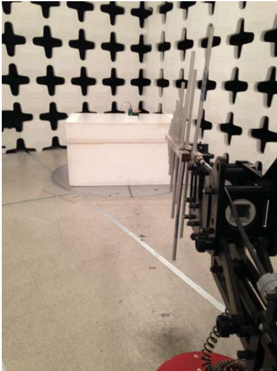
Figure 10. Radiated Spurious Emissions: 200 MHz to 1 GHz
