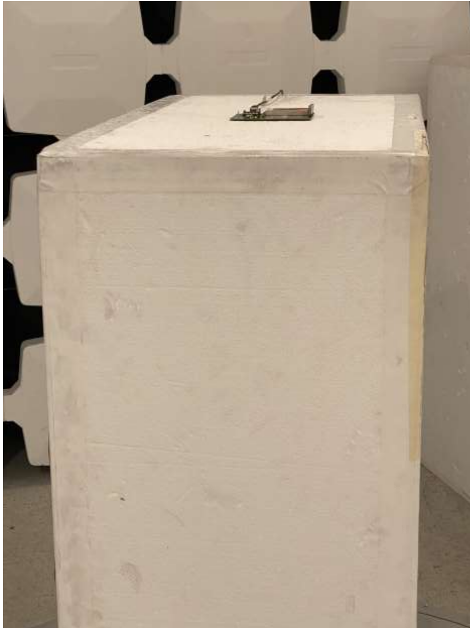
Figure 5. Radiated Emissions EUT Worst Case Position Test Setup: EUT with Patch Antenna
