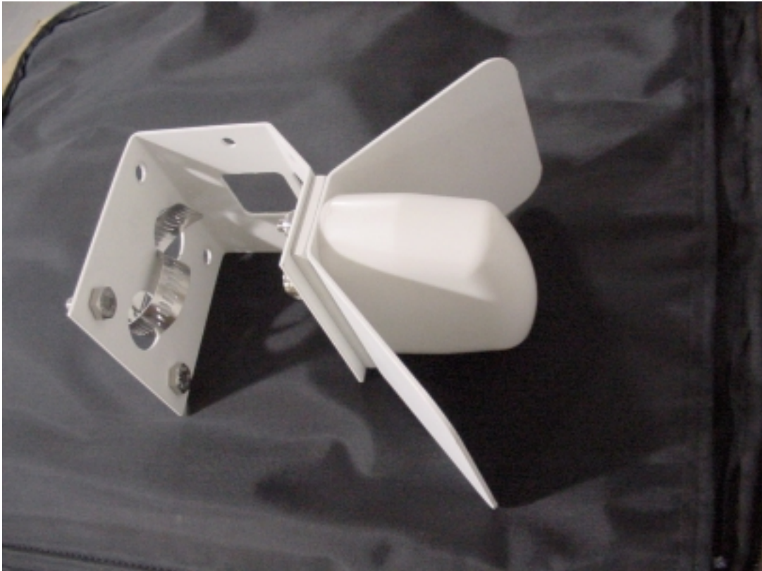
Figure 4: Mobile Mark 9dBi Corner Reflector
