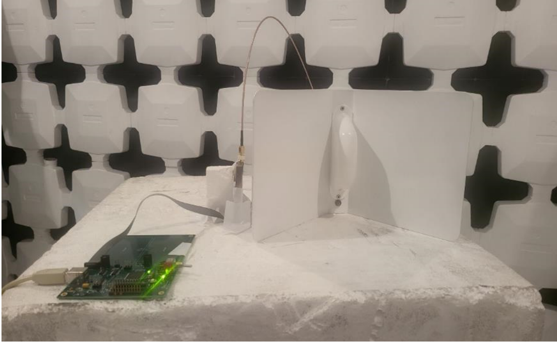
Figure 7. EUT Setup Fundamental Emissions, with Corner Reflector
