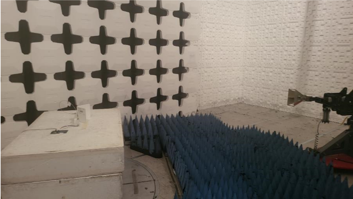
Figure 12. Radiated Emissions with Corner Reflector, above 1 GHz
