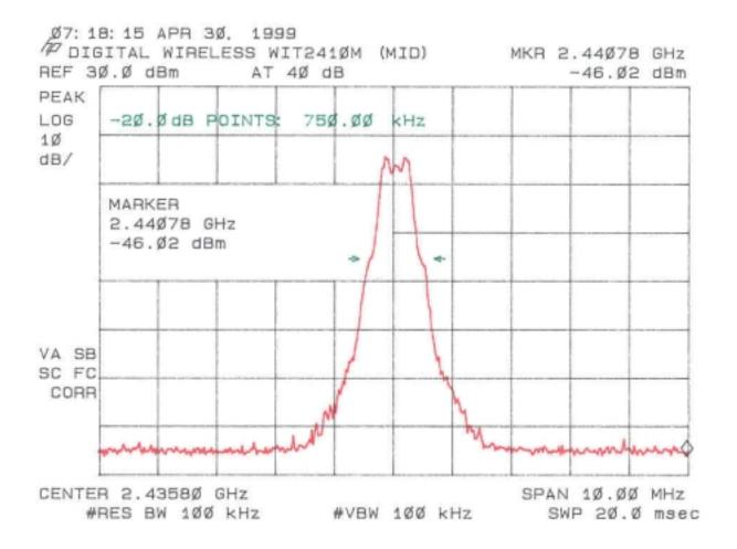
Figure 6c. 20 dB Bandwidth per FCC Section 15.247(a)(1)(ii) (High)
