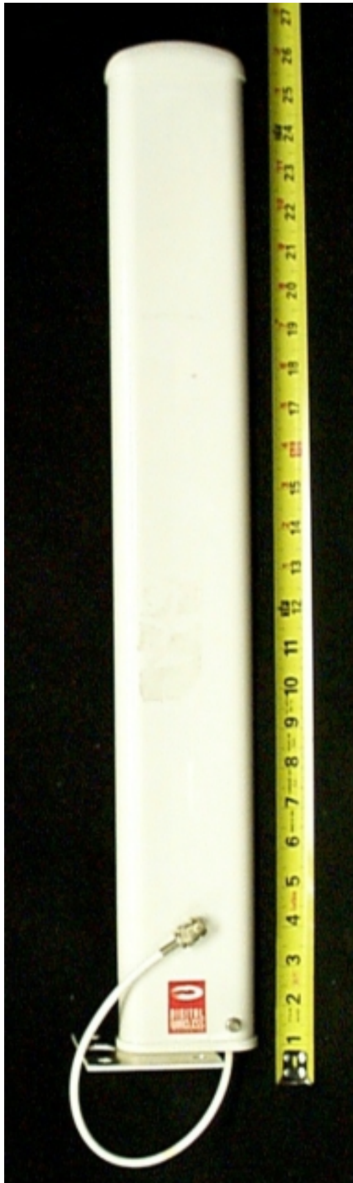
Photo 7. Antenna, Cushcraft 14 dBi Yagi (M/N PC2415-RTNF)
