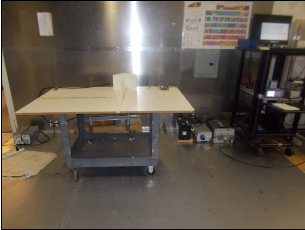
Figure 7: Conducted Emissions – Corner Antenna
