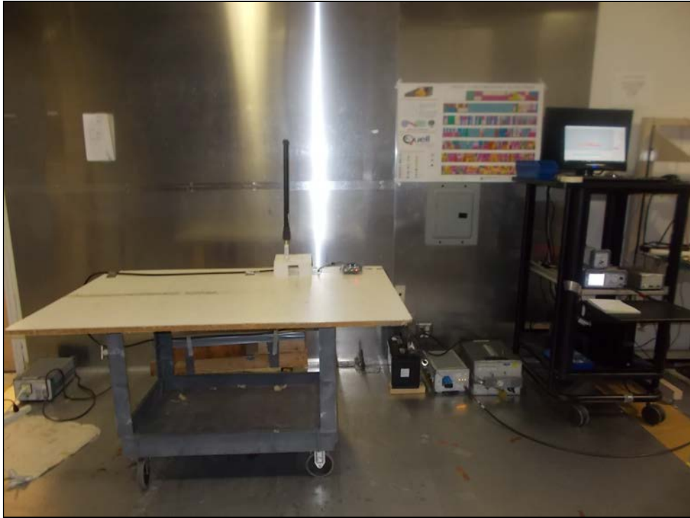
Figure 9: Conducted Emissions – Dipole Antenna
