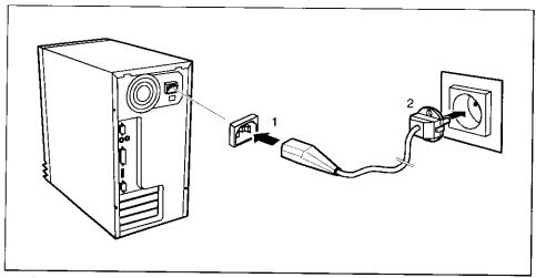
Plug the system unit's power cable into the system unit (1) and then into the grounded power outlet (2).
