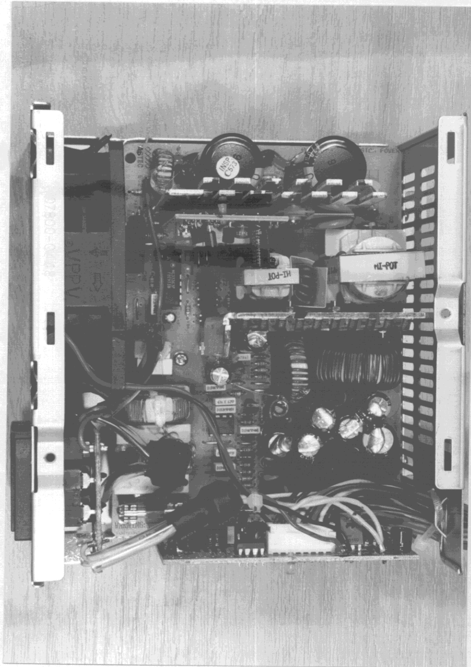
8.18 Power supply ASTEC, opened case, inside view
