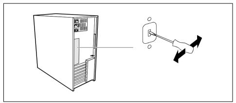
Insert a screwdriver into the opening and break out the pre-stamped installation opening by moving back and forth.
