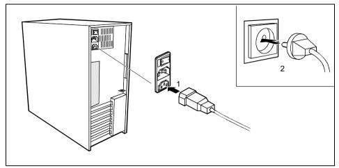
▶ Depending on the connector, plug the monitor power cable into either the system unit (1) or the grounded power outlet (2).
