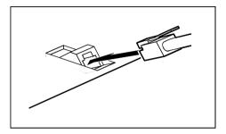
Plug the other connector of the keyboard cable into the socket on the underside of the keyboard.
