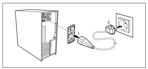
Plug the system unit's power cable into the system unit (1) and then into the grounded power outlet (2).
