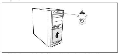
▶ Slide the drive cover in direction of the arrow (1) and turn the key clockwise (2).
