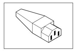
The power cord for this unit has been packed separately and has been selected for use in the appropriate country. It must be used to prevent electric shock. Use the following guidelines if it is necessary to replace the original cord set.
