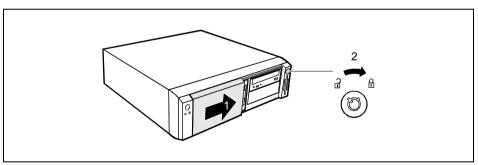
▶ Slide the drive cover in direction of the arrow (1) and turn the key clockwise (2).
