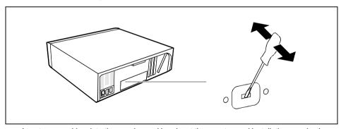
Insert a screwdriver into the opening and break out the pre-stamped installation opening by moving back and forth.
