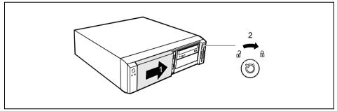
Slide the drive cover in direction of the arrow (1) and turn the key clockwise (2).
