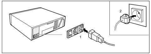
Depending on the connector, plug the monitor power cable into either the system unit (1) or the grounded power outlet (2).
