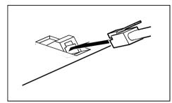
Plug the other connector of the keyboard cable into the socket on the underside of the keyboard.
