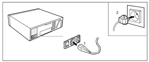
Plug the system unit's power cable into the system unit (1) and then into the grounded power outlet (2).
