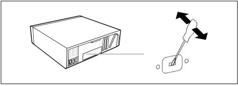
Insert a screwdriver into the opening and break out the pre-stamped installation opening by moving back and forth.
