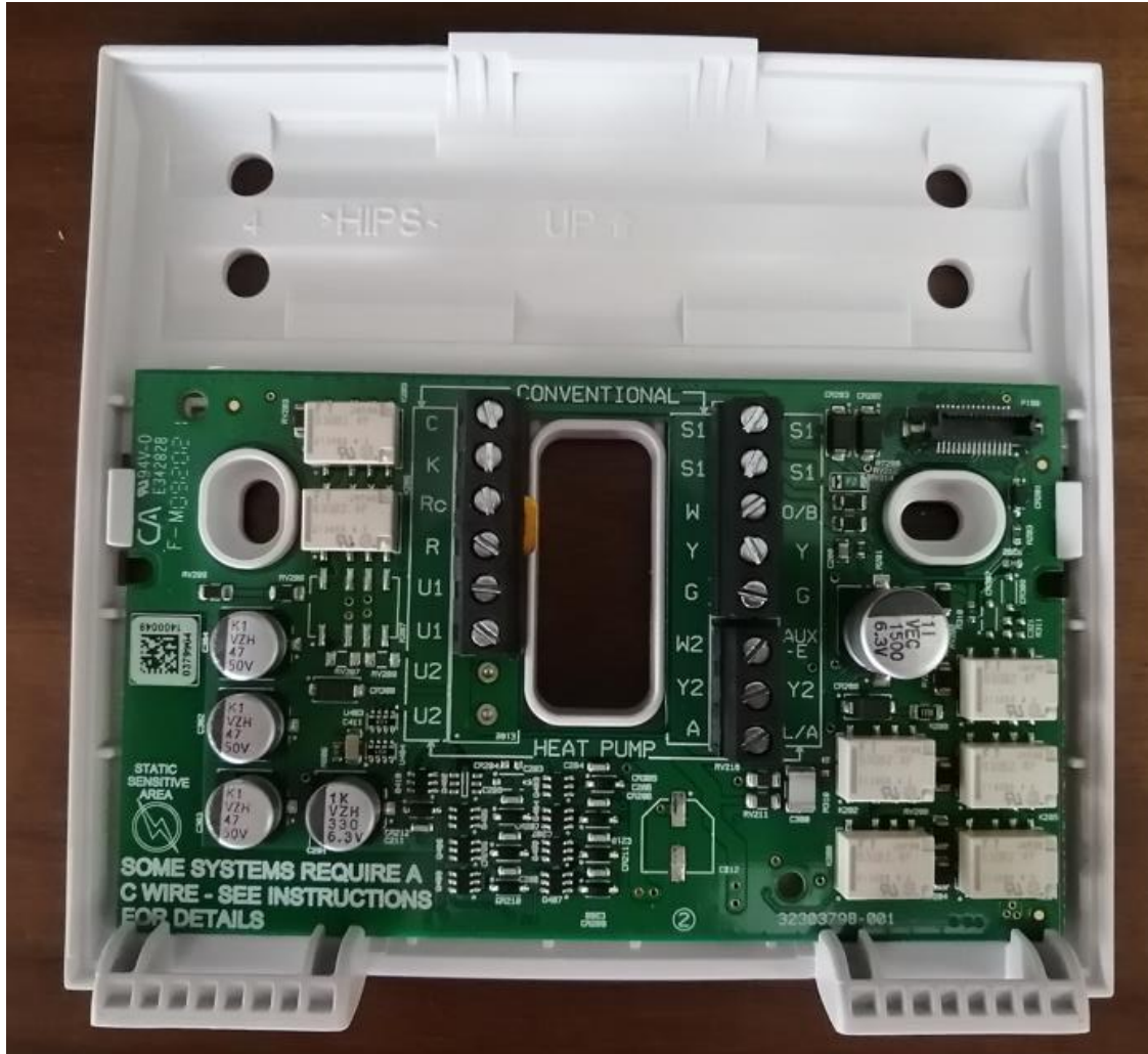
Figure 8. Wallplate front view.
