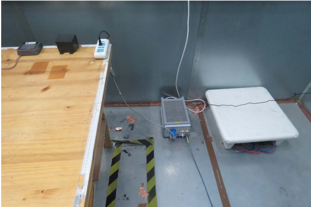
Picture 3 Conducted Emission Test Setup
