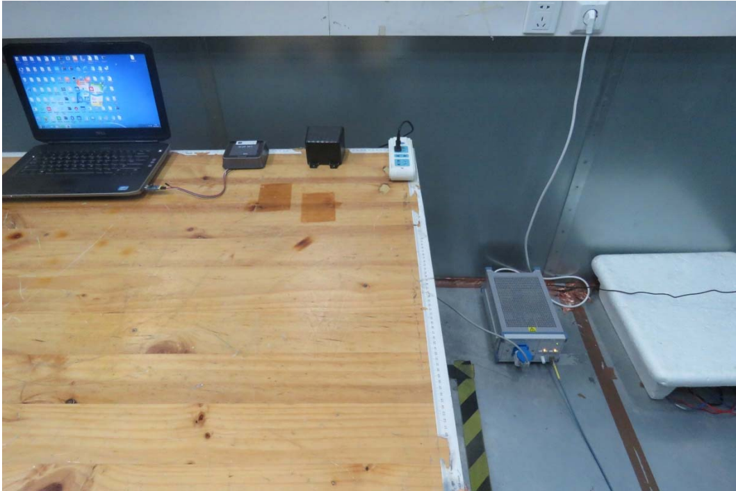
Picture 3 Conducted Emission Test Setup
