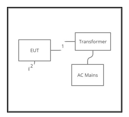
Note: Cable 2 is a UART cable used for configuration only. This cable was not populated during testing.
