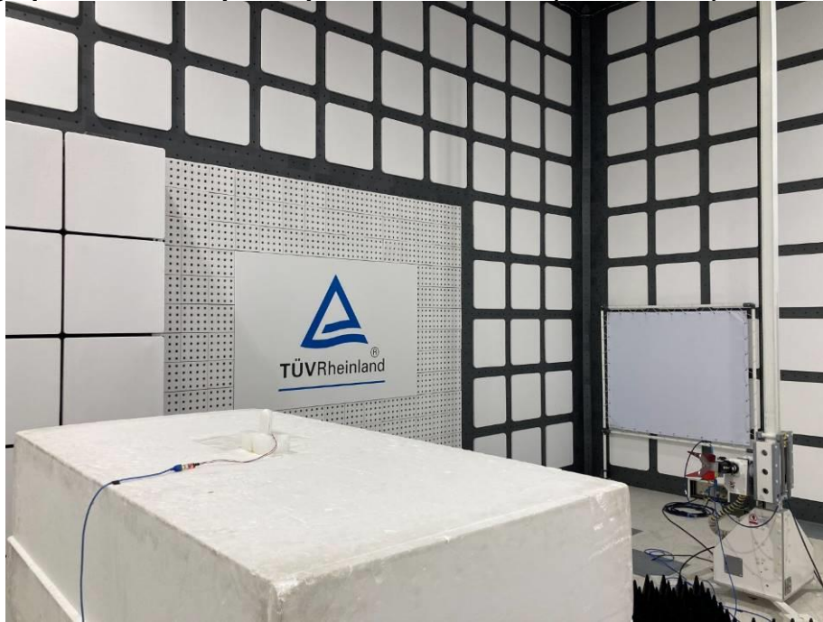
Photograph 6: Test Setup for Spurious Emissions (Back View 4)
