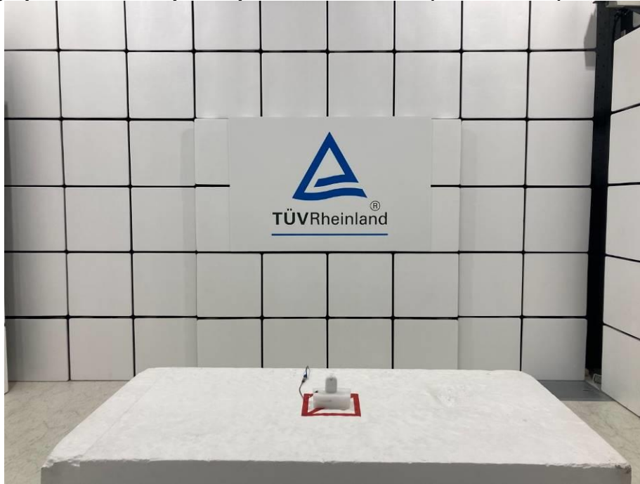
Photograph 2: Test Setup for Spurious Emissions (Front View 2)
