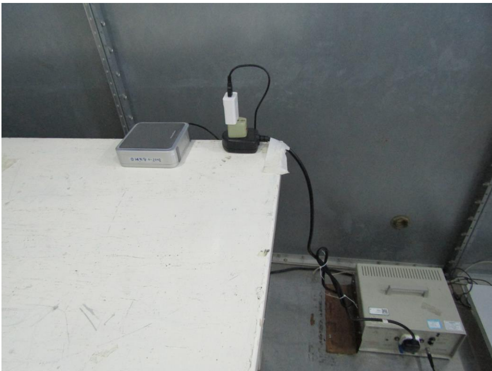
Measurement of Conducted Emission Test Set Up
