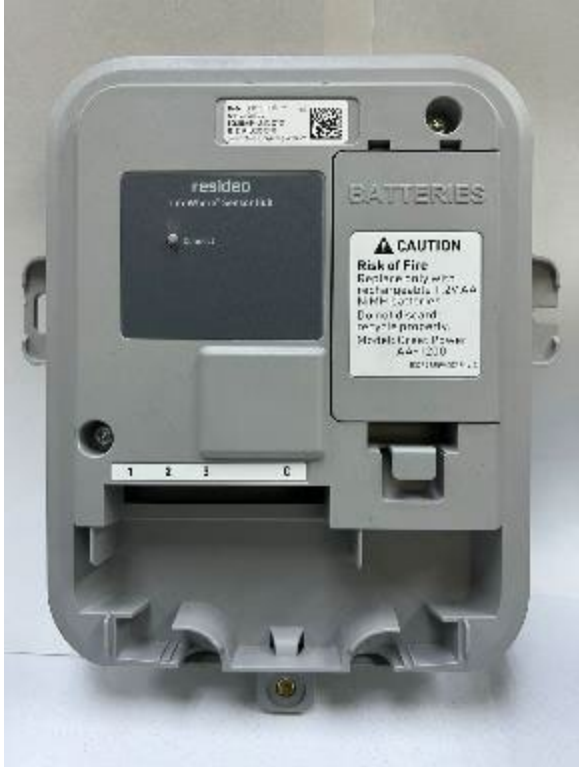
Figure 3 Assembly case back with battery compartment
