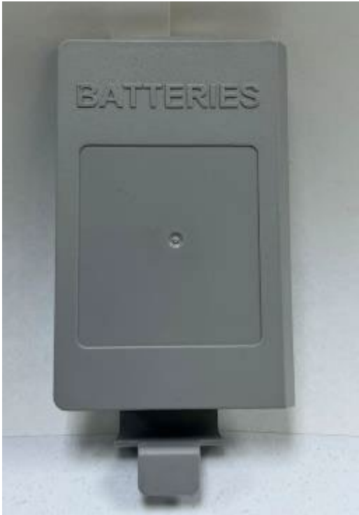
Figure 11 OSH Battery front cover without label
