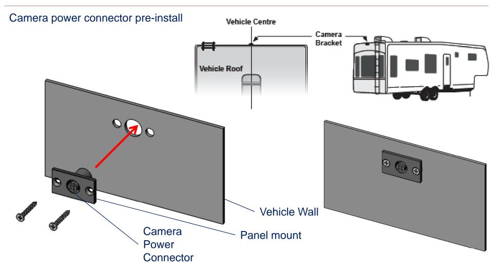
1.Camera power connector goes into the vehicle wall.2.Fix the panel mount to the rear of vehicle wall.\*The camera power connector only for WVH100 used\*
