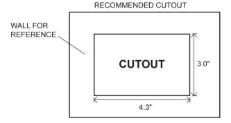
NOTE: Before cutting the mounting hole, make sure the area behind the mounting location is clear of wires, fuel and vacuum or water lines; ensure there is at least a 2.75"clearance below the Display Commander to allow for programming by USB stick.
