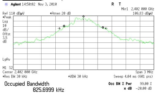
Transmit Freq Error -2.842 kHz x dB Bandwidth 852.673 kHz
