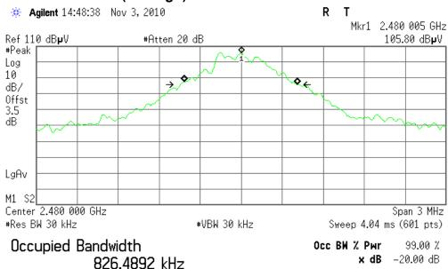
Transmit Freq Error -2.343 kHz x dB Bandwidth 848.052 kHz
