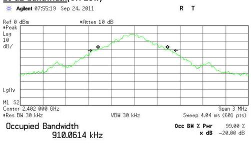
Transmit Freq Error -19.206 kHz x dB Bandwidth 974.671 kHz
