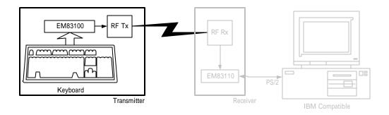
When key pressed, the keyboard control will generate a make code into FIFO and produces the digital control signals and will modulate the carrier signal. The carrier signal is generated by a crystal oscillator / frequency circuit comprised of a 27.095/27.145 MHz FSK .The frequency depend on the select channel switch to changed. The modulated output of the RF amplifier stage is coupled to the strip antenna.
