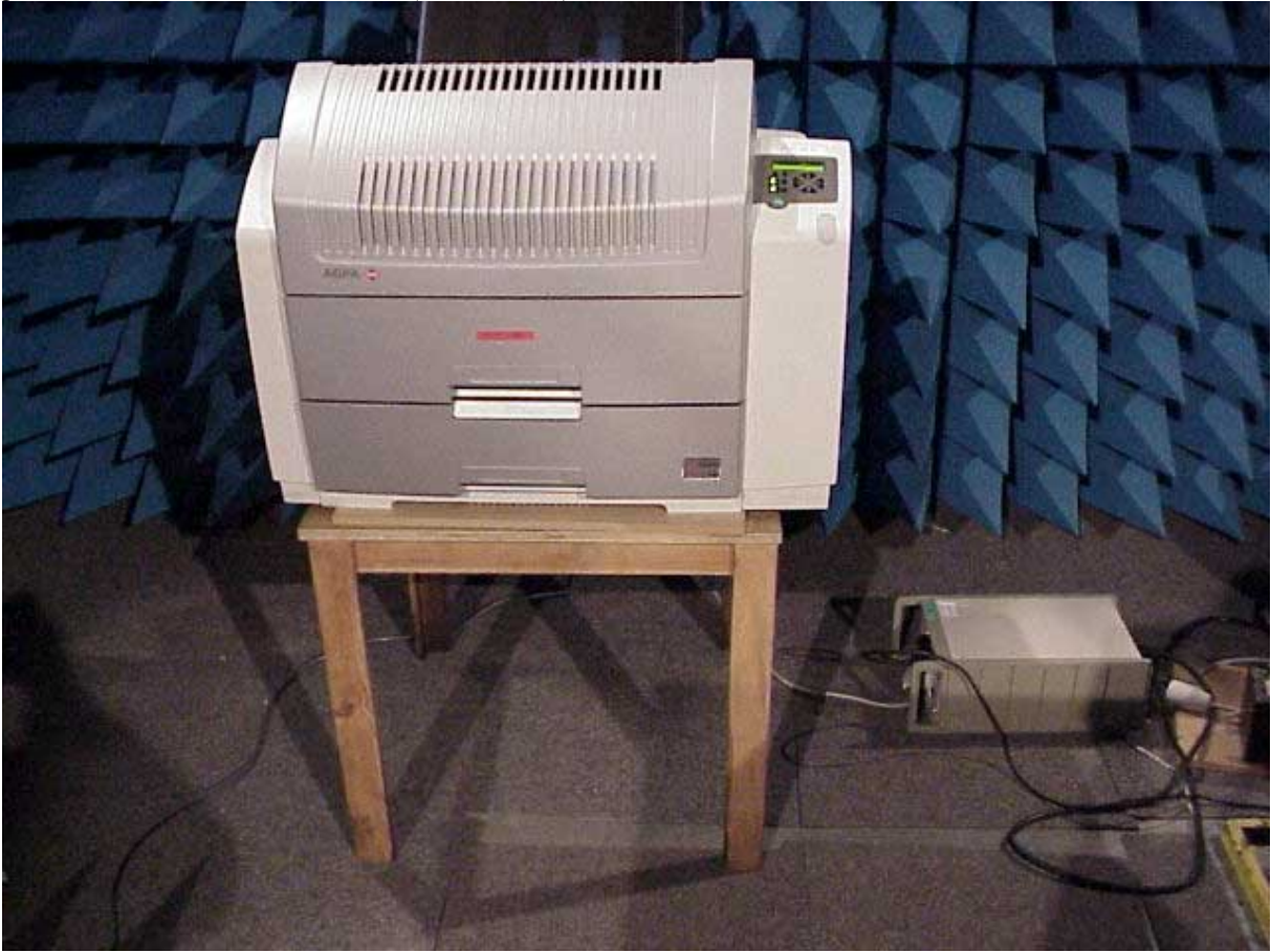
photo 1: conducted emission mains (0.15-30MHz)
