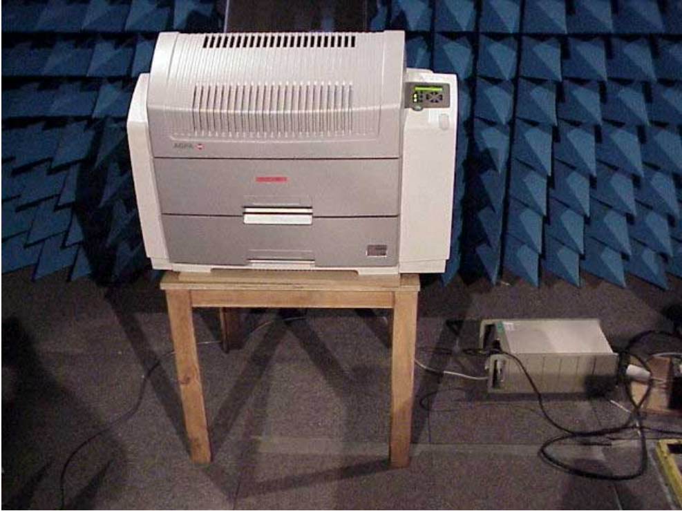
photo 2: conducted emission mains (0.15-30MHz)
