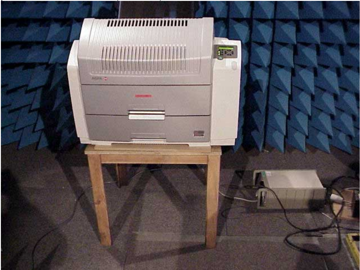
photo 6: conducted emission mains (0.15-30MHz)
