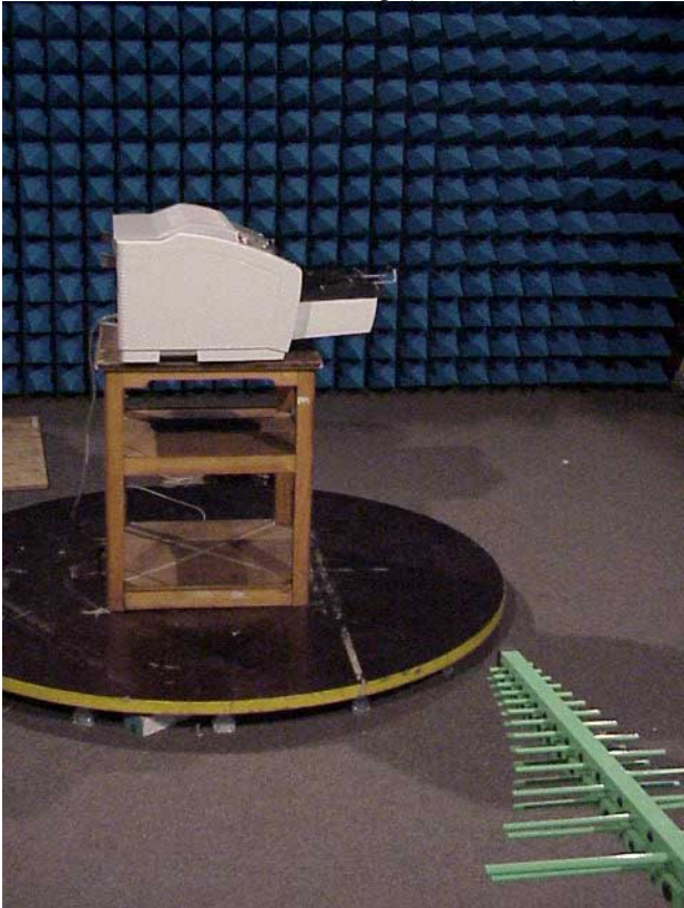
Photo 2: radiated emission set-up (30-1000MHz)
