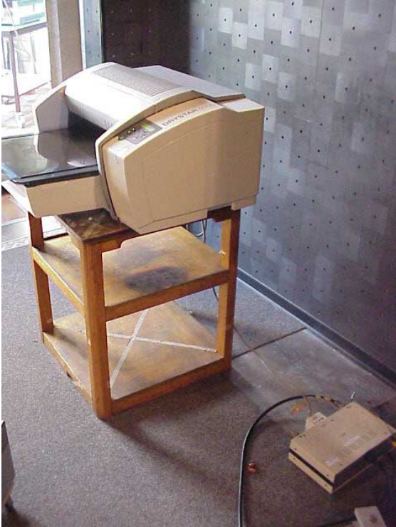
Photo 3: conducted emission mains (0.15-30MHz)
