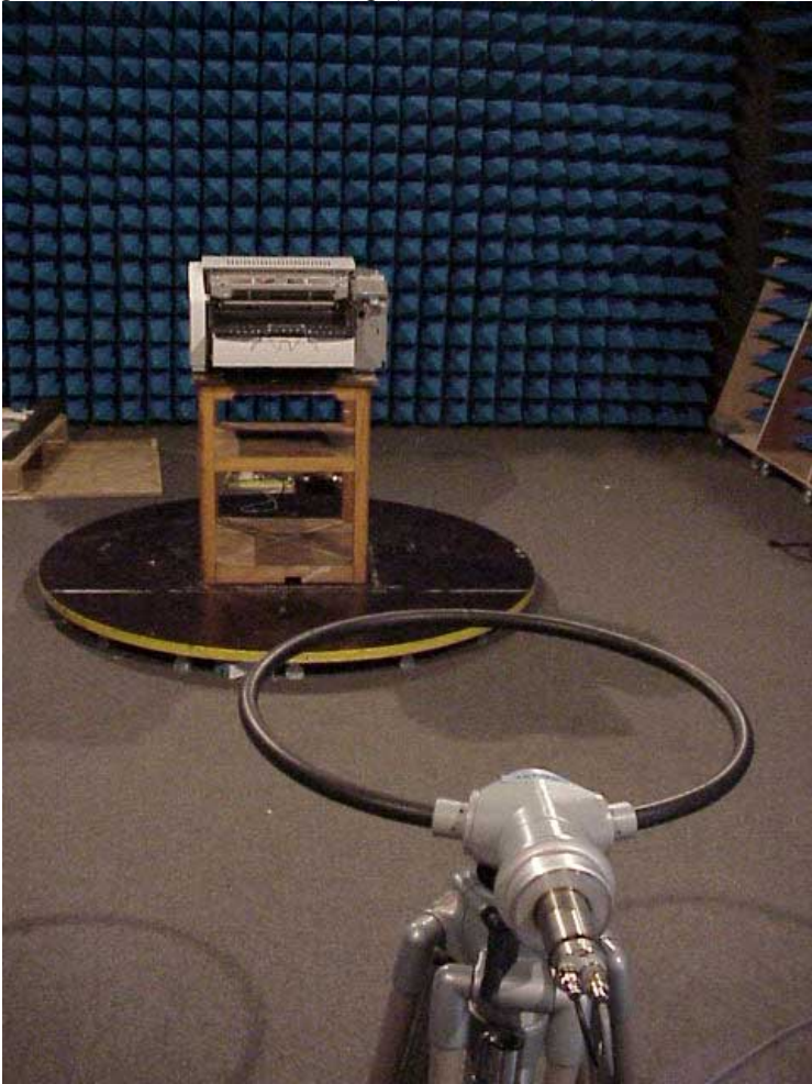
photo 5 radiated emission set-up (band 13.56MHz)
