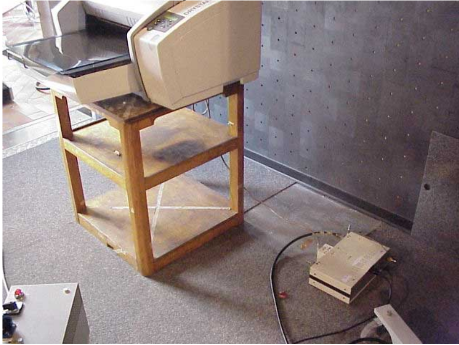
Photo 3: conducted emission set-up mains
