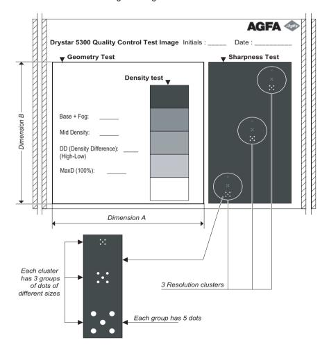
**2** To determine the reference values for geometry, measure the dimensions A and B of the geometry square on the test image.
