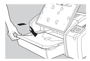
**8** Either remove the sticker completely, or leave it on the film bag; DO NOT leave it on the triangular flap!
