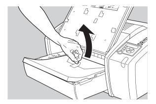
9 Slide the film pack completely into the input tray.
