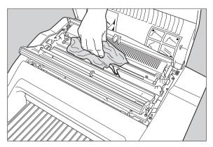
Gently pass over the resistor line a few times with a lint free cloth, slightly moistened with Isopropyl alcohol or Ethanol. **Do this only in one direction, i.e.** from left to right, without lifting the cloth.
