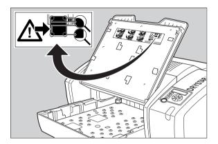
When a new film is loaded, the Film Identification tag is read and the printer settings are automatically adjusted. The Film Identification tag is located on the protective sheet on the backside of the film pack. The figure below shows the film pack upside down.
