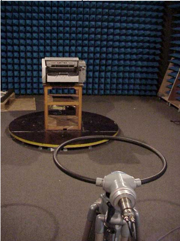
photo 5 radiated emission set-up (band 13.56MHz)
