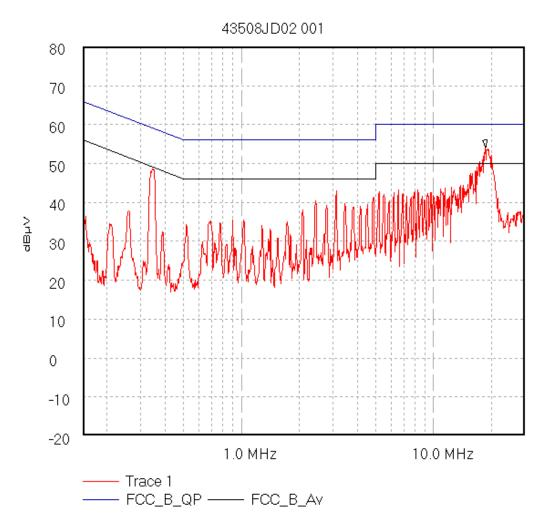
Start 150.0 kHz; Stop 30.0 MHz - Log Scale Ref 80 dBµV; Ref Offset 0.0 dB; 10 dB/div
