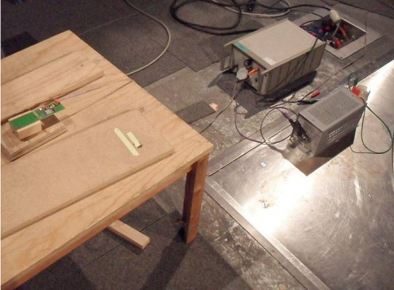
photo 1: conducted emission set-up (0.15-30MHz)
