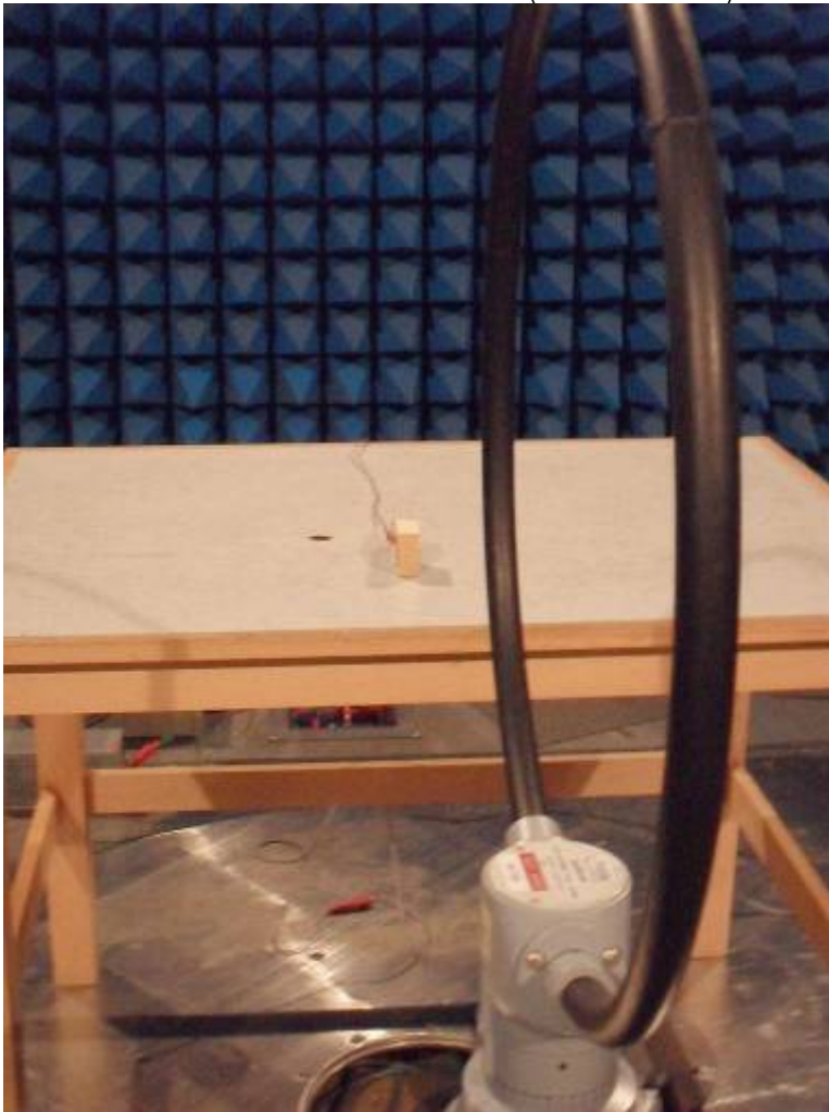
Photo 6 : fundamental radiated emission (ISM 13.65MHz)
