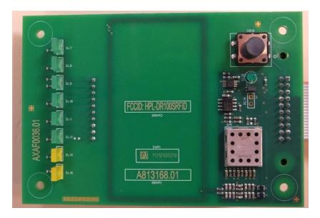
The host application will have an external, visible and permanent label that will contain the text: "Contains FCC ID: HPL-RD100SRFID"
