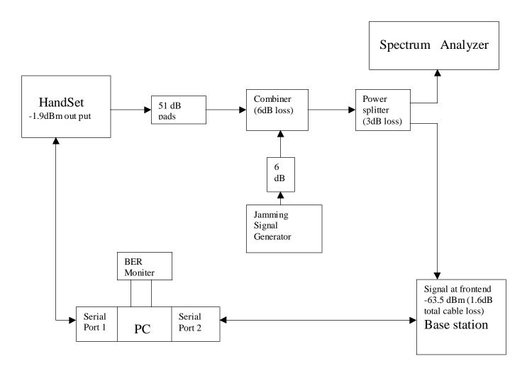
**BER** Test setup for Processing Gain measurement
