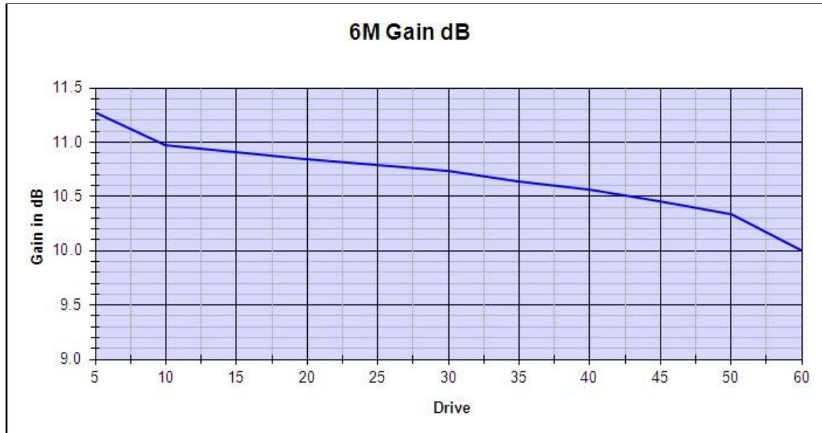
Gain vs. Drive (in watts) on highest gain band. Maximum gain is 11.3 dB. Gain remains 11.3 dB below 5 watts drive.
