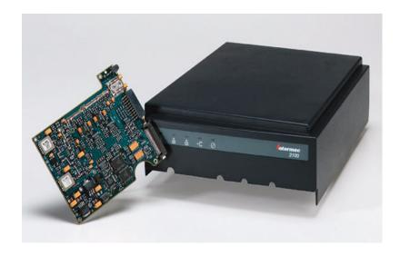
Intellitag 500 reader/programmer board sets are offered for integration into radio frequency identification (RFID) solutions requiring read range, multitag sort, read/write, and memory capacity not provided by older, less flexible proximity technology. The fixed reader/programmer board set is designed as an option to the Intermec 2100 Universal Access Point (UAP), but it may be integrated into other microcontroller-based systems.
