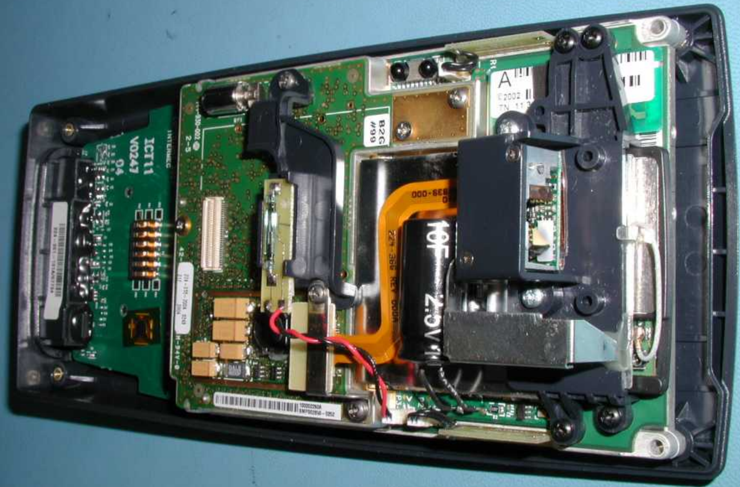
8021.. and Bluetooth modules installed in the 700C. (802.11 protective cover removed)
