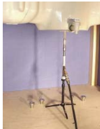
1800MHz System Check Setup
