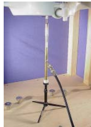
2450MHz System Check Setup
