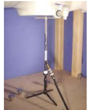
900MHz System Check Setup
