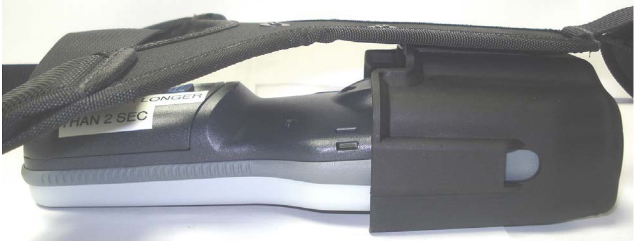
Left Side of CK31 Hand-held PC (Small Back) with Holster accessory (P/N: 825-169-001)
