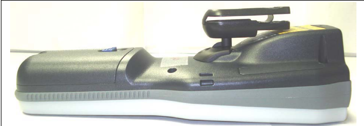
Left Side of CK31 Hand-held PC (Large Back) with Swivel Belt-Clip accessory
