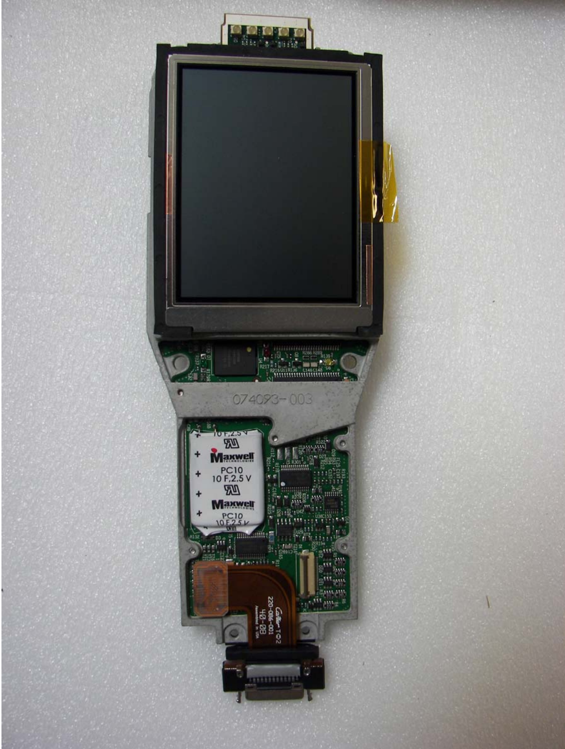
CK31 – front view. Front enclosure removed.
