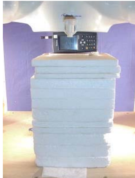
SAR Test Setup Right Side of EUT
