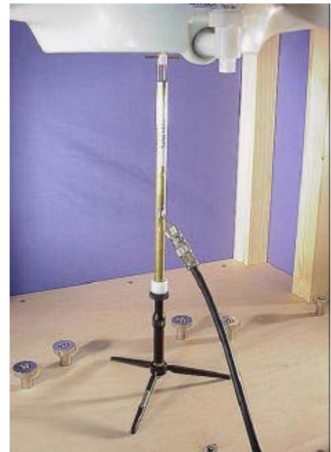
2450MHz Dipole Validation Setup
