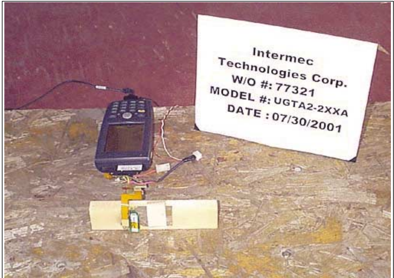
Radiated Emissions - Orthogonal B Front View Close-up
